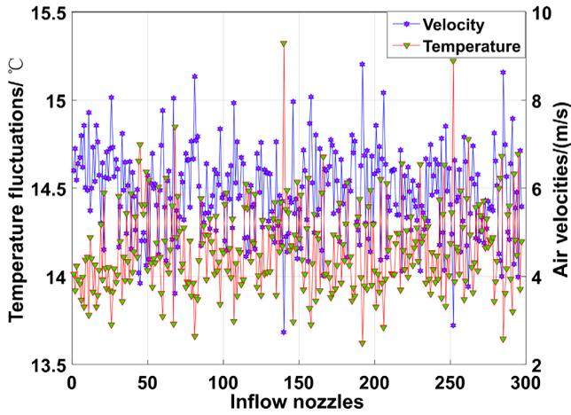
**Fig. 10** The air flow velocities of 297 INs (blue line) and the produced temperature differences on the mirror surface (red line) ( $\sigma_V = 1$  m/s,  $\sigma_{\Delta T} = 0.24^\circ\text{C}$ ).
