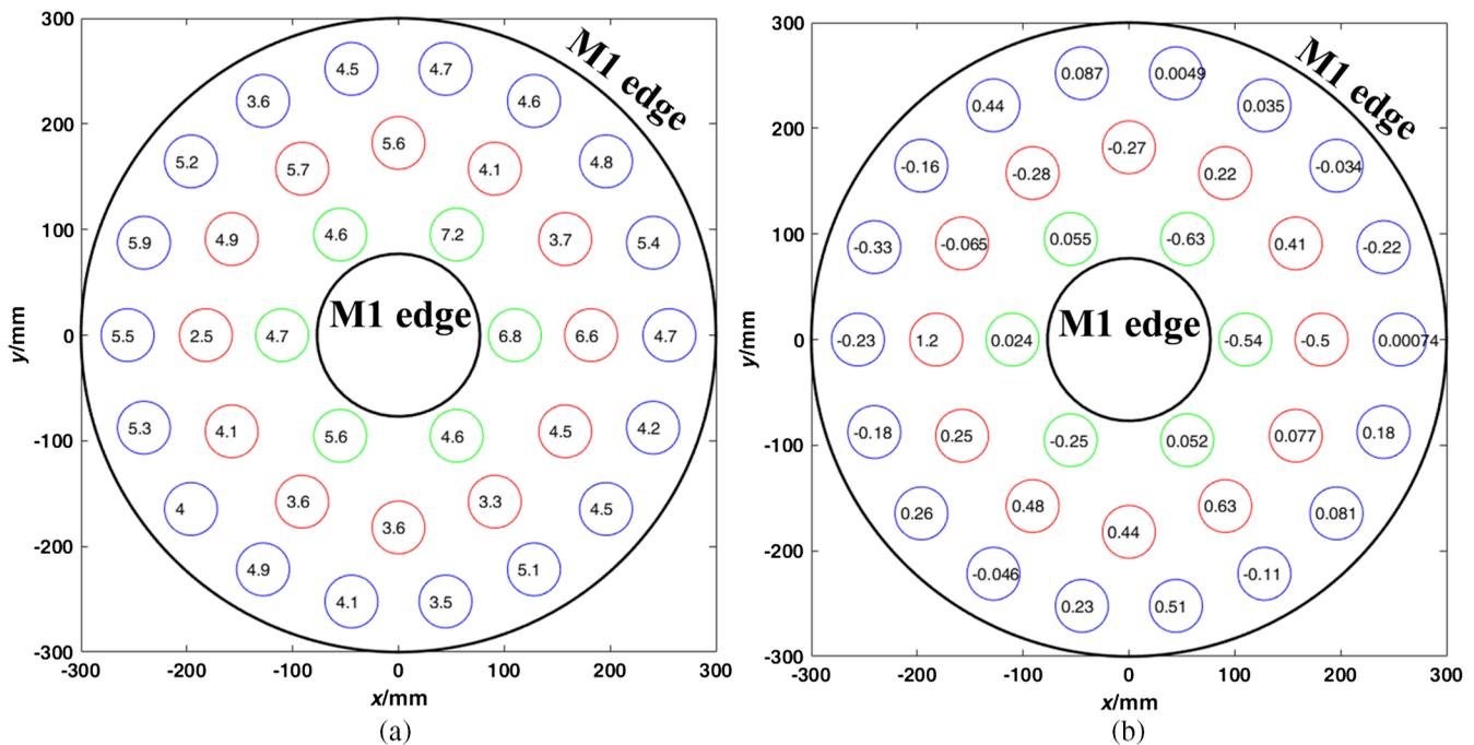
**Fig. 4** A random set of air flow velocities and its influence on the temperature of the mirror surface. (a) The air flow velocities of 36 INs. (b) The influence on the temperature of the mirror surface.
