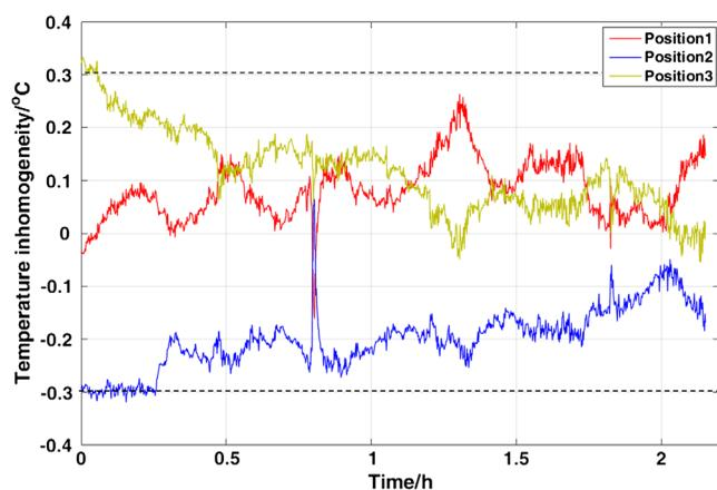
Fig. 8 The recorded temperature values on three positions of the mirror surface and their differences.
