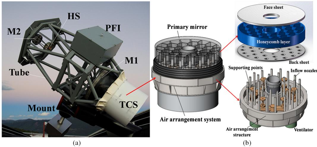
**Fig. 3** A picture of (a) the POST and (b) a sketch map of its TCS structure. M1, the primary mirror; M2, the secondary mirror; M3, the fold mirror; HS, the heat stop; PFI, the postfocus instruments; TCS, the thermal control system.
