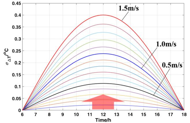
**Fig. 11** The standard deviation values of the temperature differences during daytime with different  $\sigma_V$  values.
