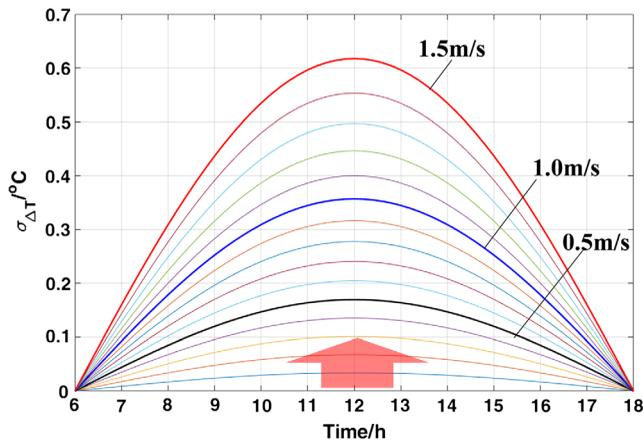
Fig. 5 The standard deviation values of the temperature differences during daytime with different  $\sigma_V$  values.
