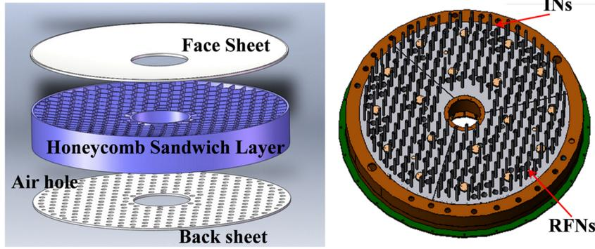
**Fig. 9** The light-weighted honeycomb primary mirror and its air arrangement system (IN, inflow nozzle; RFN, return flow nozzle).
