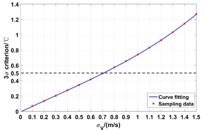
**Fig. 12** The  $3\sigma$  criterion of the temperature differences across the mirror surface with different  $\sigma_V$  values (CLST).
