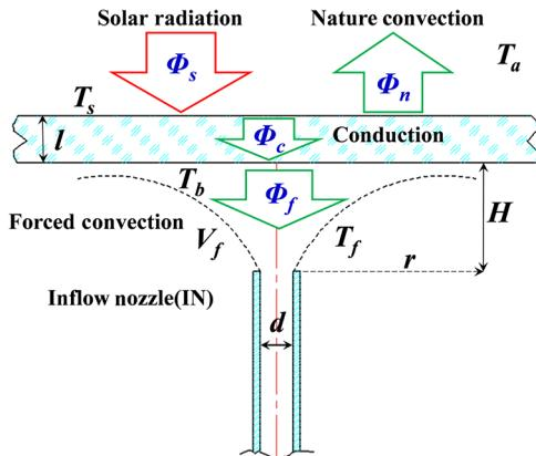
**Fig. 1** Illustration of the cooling process of an air flow.  $T_s$ , temperature of the mirror surface;  $T_b$ , temperature of the back of the face sheet;  $T_a$ , temperature of the ambient air;  $d$ , in-circle diameter of the IN;  $H$ , distance from the INs tip to the bottom of the face sheet;  $l$ , thickness of the face sheet.
