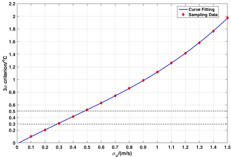
Fig. 6 The  $3\sigma$  criterion of the temperature differences on the mirror surface with different  $\sigma_V$  values (POST).
