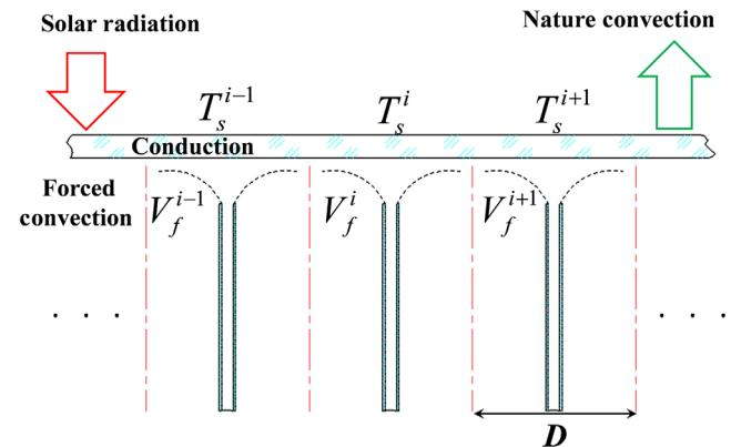
**Fig. 2** Illustration of the differences between the air flow velocities of the INs, and the influence on the temperature of the mirror surface at associate positions.  $V_f^i$ , air flow velocity at the tip of the  $i$ 'th IN;  $T_s^i$ , temperature of the mirror surface at the  $i$ 'th IN.
