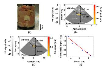
**Fig. 4** PA imaging of a MB-containing tube in chicken tissue. MB, methylene blue. (a) Photograph of the sample setup. (b) Overlaid PA and US image of the tube at 3.4 cm depth. (c) Overlaid PA and US image of the tube at 8.4 cm depth. (d) PA signal (normalized by the signal at the smallest depth) as a function of depth. The maximum depth is 8.4 cm. SNR at this depth is 5.6 (15 dB). The 1/e penetration-depth based on linear curve-fitting is 1.11 cm.
