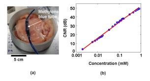
**Fig. 6** PA signal strength as a function of methylene blue concentration at a depth of 3.4 cm measured using the S5-1 probe. (a) Photograph showing the methylene blue tube embedded in chicken breast tissue. The methylene blue tube was covered by 3.5 cm of chicken breast tissue during PA imaging. (b) CNR versus concentration after subtraction of the baseline signal.
