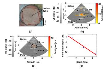
**Fig. 5** TA imaging of saline tube in pork fat tissue. (a) Photograph showing the saline tube embedded in fat tissue. The saline tube was buried under additional layers of fat tissue during TA imaging. (b) TA and US overlaid image at a depth of 1.1 cm. (c) TA and US overlaid image of the tube at a depth of 4.4 cm (in the dotted frame). (d) TA signal (normalized by the signal at the smallest depth) as a function of depth. The maximum depth is 4.4 cm. SNR at this depth is 5.7 (15.1 dB).
