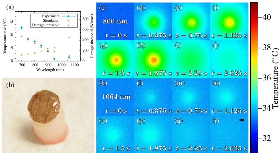
**Fig. 2** (a) Temperature rise measured as a function of excitation wavelength. Simulated temperature rise and estimated damage thresholds are also displayed. (b) Tissue sample used for laser-induced heating measurements. (c)–(j) Subset of thermal images for 800-nm excitation. (k)–(r) Subset of thermal images for 1064-nm excitation. A 200- $\mu\text{m}$  scale bar is included in (r).
