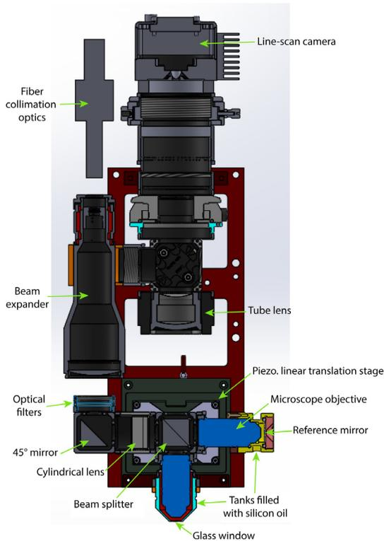
**Fig. 2** Construction plan of the LC-OCT imaging head.
