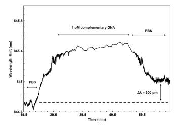
Fig. 3 Wavelength shift due flow of 1 pM complementary DNA on the sensor.
