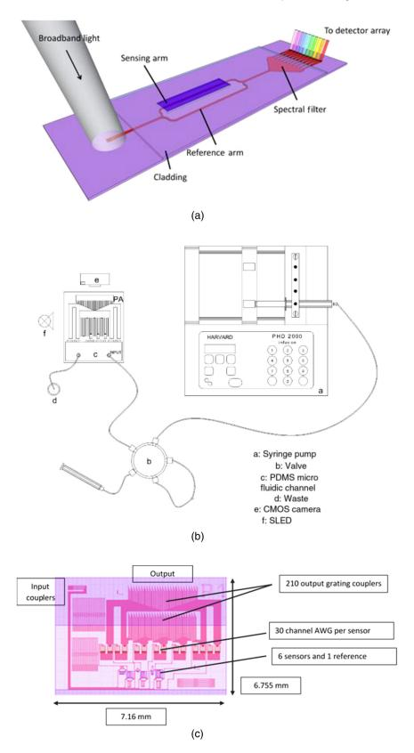
**Fig. 1** (a) Schematic of the optical setup used for the DNA detection, (b) schematic of the experimental setup, and (c) photonic integrated circuits (PICs) sensor.
