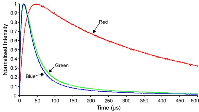
**Fig. 7** Phosphor intensity versus time response for the three phosphors of a typical cathode ray tube (CRT) display.<sup>46</sup>
