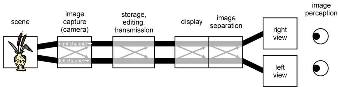
**Fig. 3** A flow diagram showing the transfer of stereoscopic images from image capture through to image viewing and perception by the observer. Crosstalk between the left and right image channels can occur in the capture (camera) stage, storage/editing/transmission stage, image display (light generation), and image separation (3D glasses or autostereoscopic optical layer) stages. Most crosstalk usually occurs in the display and image separation stages.
