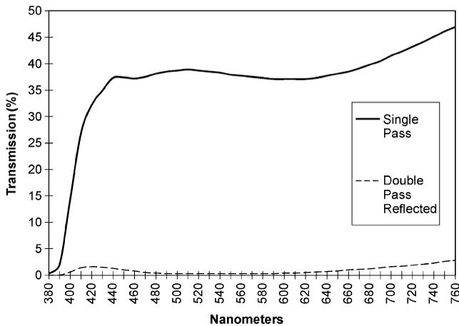
**Fig. 16** Spectral response of single and “crossed” circular polarizers.<sup>64</sup> The dashed curve is a representation of the amount of leakage that will occur between two circular polarized channels of a polarized stereoscopic display due exclusively to the polarization quality of the polarizers.
