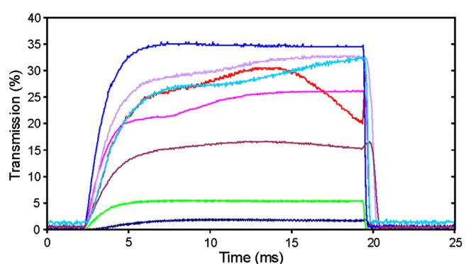
**Fig. 5** The transmission versus time response of a selection of different LCS glasses at green wavelengths (measured using a green LED continuous light source). There can be a wide variability of performance between different shutter glasses.<sup>46</sup>
