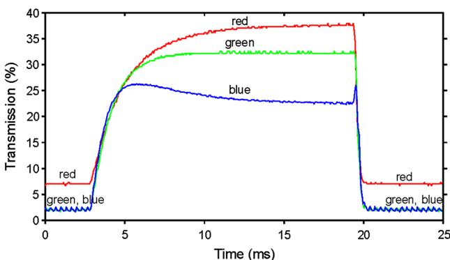
**Fig. 4** The transmission versus time response of an example pair of active shutter glasses at red, green and blue wavelengths (measured using red, green and blue light emitting diode (LED) continuous light sources).<sup>46</sup>
