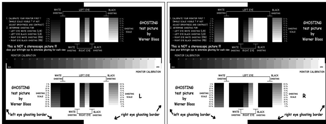
Fig. 23 Crosstalk measurement test chart designed by Bloos.<sup>104</sup>
