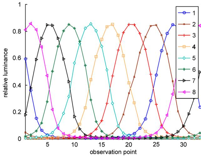
**Fig. 20** The visibility of different perspective views as output by an example lenticular multi-view autostereoscopic display when viewed from different horizontally spaced observation points.<sup>80</sup> For example, from viewing position (observation point) 20, view 3 is dominant, but some of views 2 and 4 are also visible which causes crosstalk. This figure shows severe crosstalk for illustrative purposes and is not intended to be representative of all modern autostereoscopic displays.
