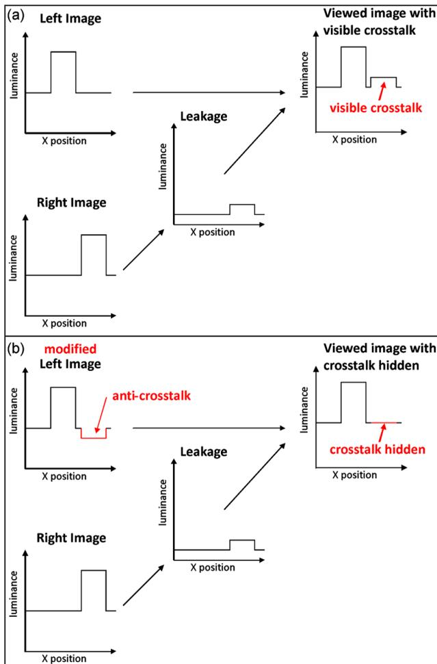
**Fig. 24** A simple illustration of the process of crosstalk cancellation on a stereoscopic display. (a) An example of a stereoscopic image with crosstalk visible to the left eye from the leakage of light from the right image channel. (b) An example of anti-crosstalk being applied to the left image so that when leakage occurs from the right image channel, it cancels with the anti-crosstalk to hide the crosstalk.
