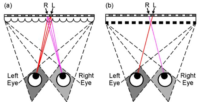
**Fig. 19** Example configuration of (a) two-view lenticular autostereoscopic display and (b) two-view parallax barrier autostereoscopic display (top view). The optical elements ideally act to allow the left eye to see only the left image pixels, and the right eye to only see the right image pixels. The 'sweet spots' where this optical isolation works best are shown in gray.
