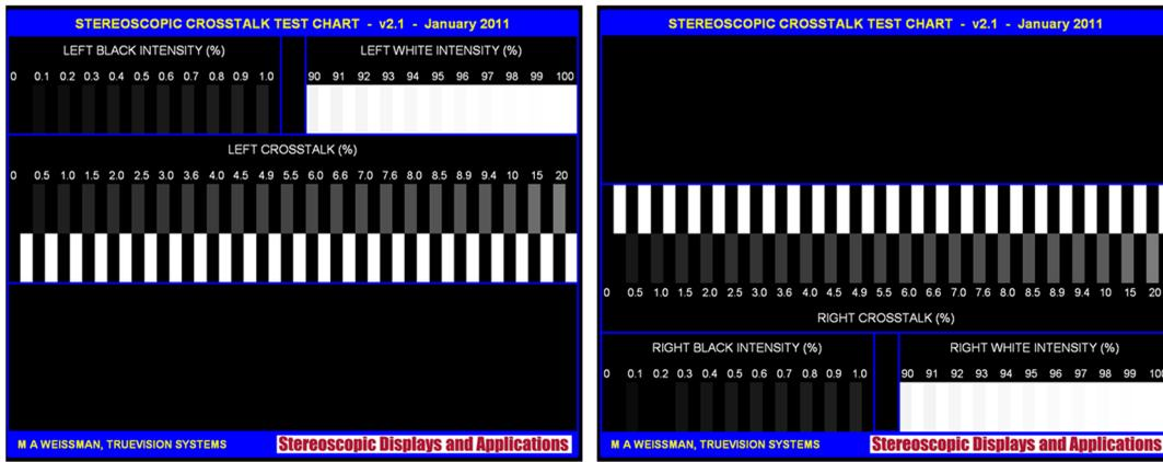
Fig. 22 Crosstalk measurement test chart designed by Weissman.<sup>103</sup>
