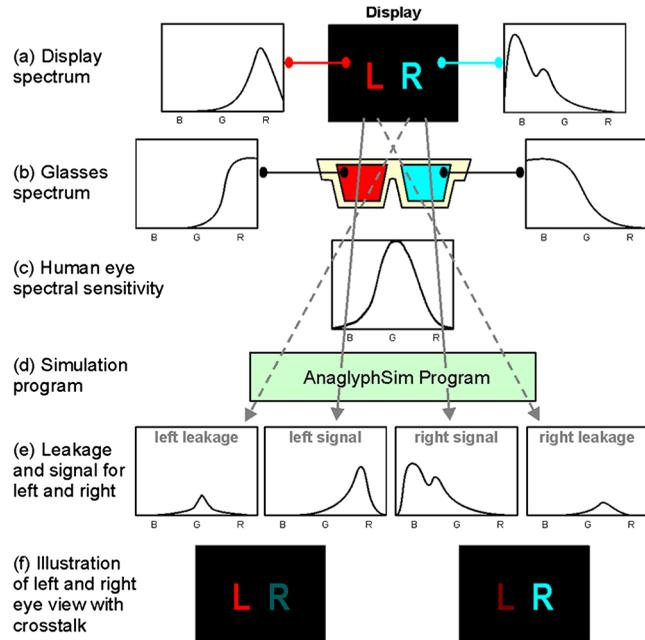
**Fig. 21** Illustration of the process (and simulation) of crosstalk in anaglyph 3D displays. From the top: (a) Spectral response of display, (b) spectral response of anaglyph glasses, (c) human eye spectral sensitivity, (d) simulation of crosstalk using a computer program, (e) spectral output characteristic of crosstalk and intended image, and (f) visual illustration of left eye and right eye view with crosstalk.<sup>15</sup>
