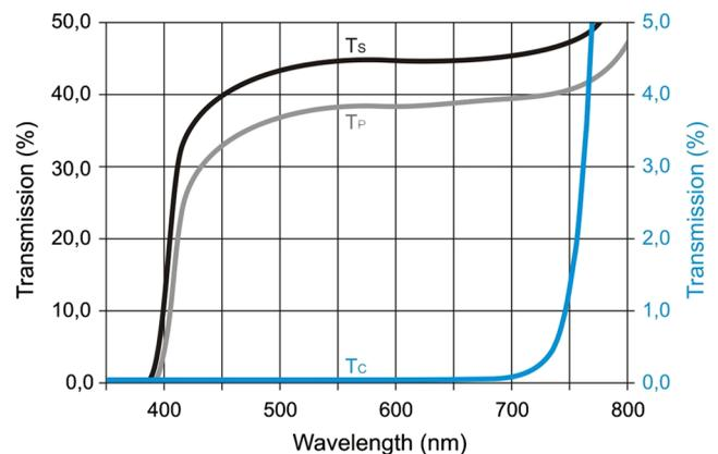
**Fig. 15** Spectral response of an example linear polarizer in single  $T_s$ , parallel  $T_p$  and crossed  $T_c$  configurations.<sup>63</sup> The blue “crossed” curve is a close approximation of the amount of leakage that will occur between two linear polarized channels of a polarized stereoscopic display (excluding the effect of head tilt and screen depolarization).
