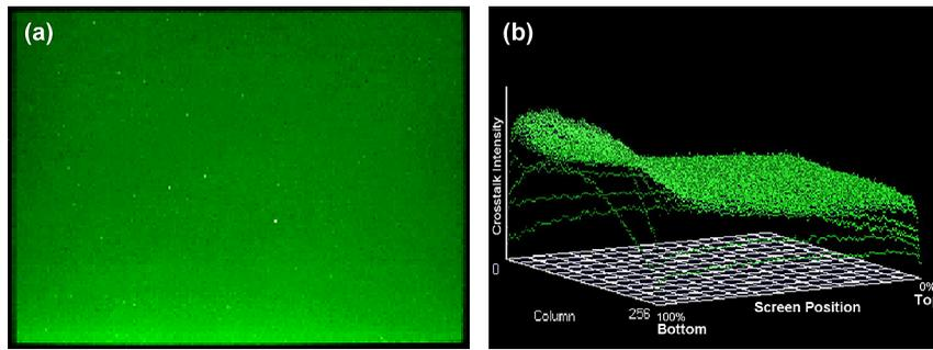
**Fig. 9** Illustration of spatial variation of crosstalk on a cathode ray tube (CRT), with increased crosstalk at the bottom of the screen: (a) actual screen photograph of CRT crosstalk through a pair of active shutter glasses, and (b) histogram of measured CRT crosstalk.<sup>46</sup>
