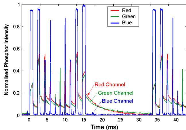
**Fig. 10** The time-domain light output of an example plasma display (showing alternating frames of 100% white and black). The vertical axis is the normalized phosphor intensity.<sup>47</sup> This graph illustrates the 10 pulses per frame used to construct images with various gray levels and the long phosphor persistence of the red and green channels (of this particular display).
