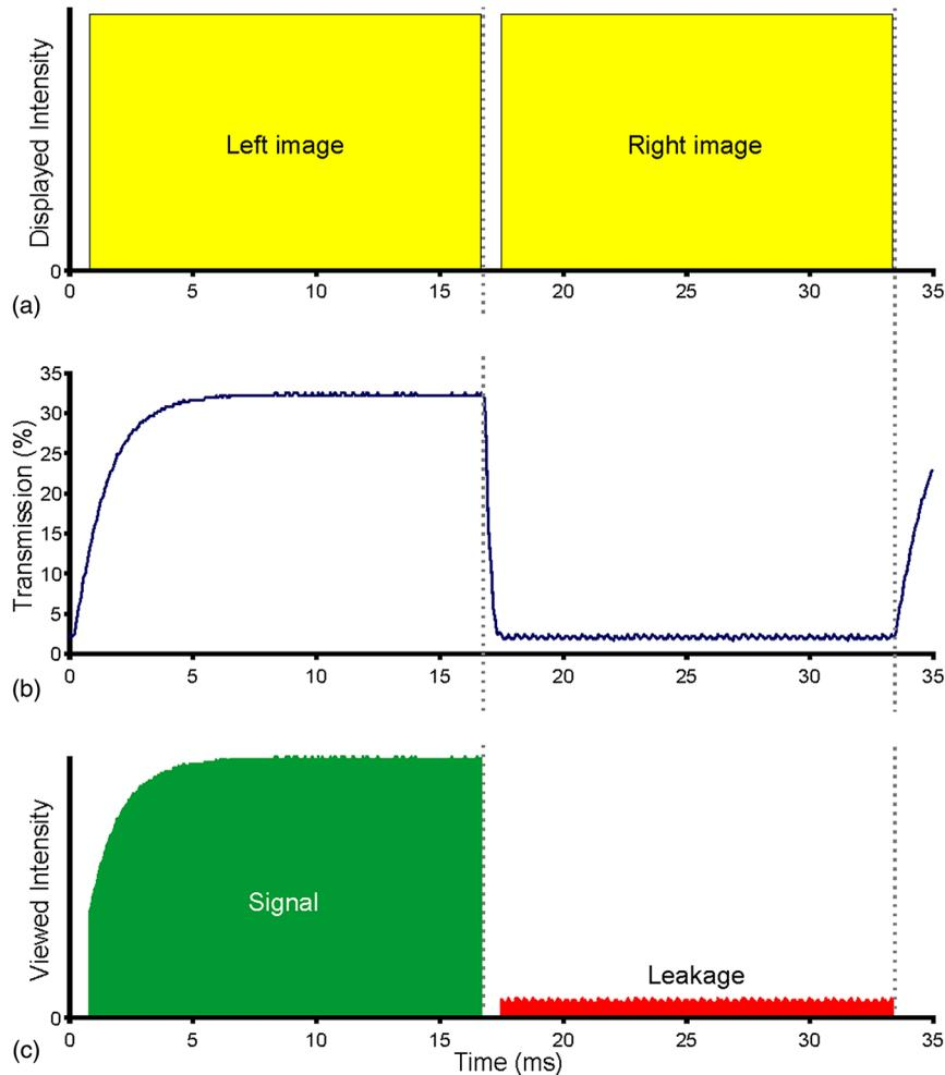
**Fig. 6** An illustration of how a pair of shutter glasses interacts with the left/right image sequence of a theoretical time-sequential stereoscopic display. (a) The sequence of left and right images output by a theoretical display with instantaneous pixel response. (b) The transmission versus time of the left-eye LC shutter. (c) The image intensity as viewed through the left-eye of the LC glasses.
