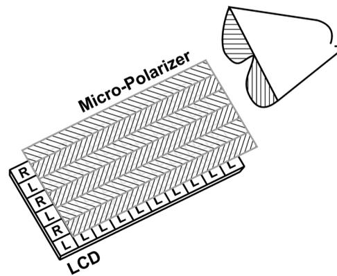
**Fig. 17** The optical layout of a micro-polarized 3D LCD. A micropolarizer layer over the front of the LCD polarizes alternate rows of pixels into two different polarization states.<sup>73,74</sup> In this example an observer wearing a pair of polarized 3D glasses will see the odd-numbered rows of pixels through the right eye, and the even-numbered rows of pixels through the left eye.
