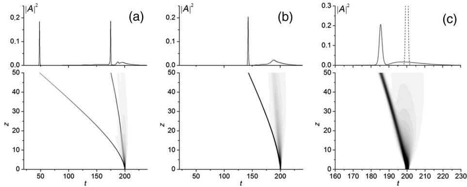
**Fig. 10** Maximal intensity position for both subpulses at the incident Gaussian pulse propagation for the positive phase amplitude grating (a)  $\xi = 5$ , (b) 2.5, (c) 1 and  $\delta_0 = 0.05$ ,  $\tilde{\delta} = 5$ . The top figures show subpulse shapes at section  $z = 50$ . Dashed line in top figure (c) shows the incident pulse shape.
