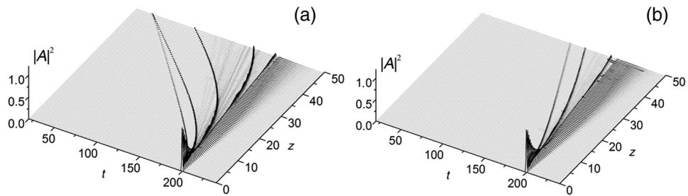
**Fig. 12** Soliton formation at the incident Gaussian pulse propagation in the medium with parameters  $\delta_0 = 0.05$ , (a)  $\xi = 2.5$ , (b) 1.25, and  $\bar{\delta} = 5$ .
