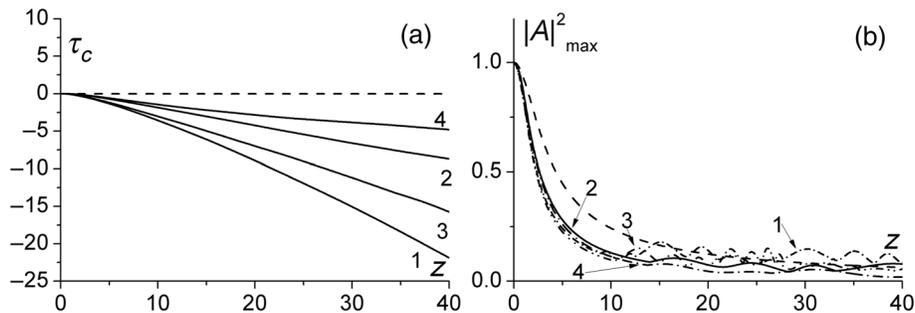
**Fig. 11** (a) Pulse center shifting along the  $z$ -coordinate, calculated using Eq. (12) and (b) maximal intensity evolution for the positive phase amplitude grating and  $\delta_0 = 0.05$  (curves 1 and 2), 0.1 (curves 3 and 4),  $\xi = 2.5$  (curves 1 and 3), 1.25 (curves 2 and 4), and  $\tilde{\delta} = 5$ . Dashed lines correspond to the pulse propagation in a linear medium.
