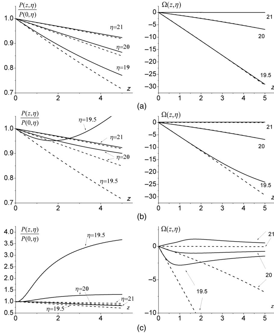
**Fig. 3** Temporal integral of the optical pulse intensity  $P(z, \eta)$  and instantaneous frequency  $\Omega(z, \eta)$  evolution along the characteristics for the three values of  $\eta$  (indicated by figures) at the incident Gaussian pulse propagation in a medium with SPA and (a)  $D = 10^{-4}$ , (b)  $10^{-3}$ , (c) 0.1,  $\xi = 5$ ,  $\delta_0 = 0.05$ , and  $\tilde{\delta} = 5$ . Dashed lines correspond to the curves obtained using Eqs. (17), (20), and (23).
