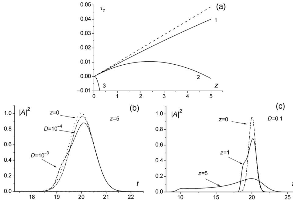
**Fig. 4** (a) Pulse center shift evolution for the incident Gaussian pulse propagation in a medium with SPA and (1)  $D = 10^{-4}$ , (2)  $10^{-3}$ , (3)  $0.1$ ; dashed line corresponds to the curve obtained using Eq. (21); (b) pulse shapes at  $z = 0$  (dotted line),  $5$  for  $D = 10^{-4}$  (dashed-dotted line),  $10^{-3}$  (solid line); (c) pulse shapes at different sections for  $D = 0.1$ ; other parameters are  $\xi = 5$ ,  $\delta_0 = 0.05$ ,  $\tilde{\delta} = 5$ .
