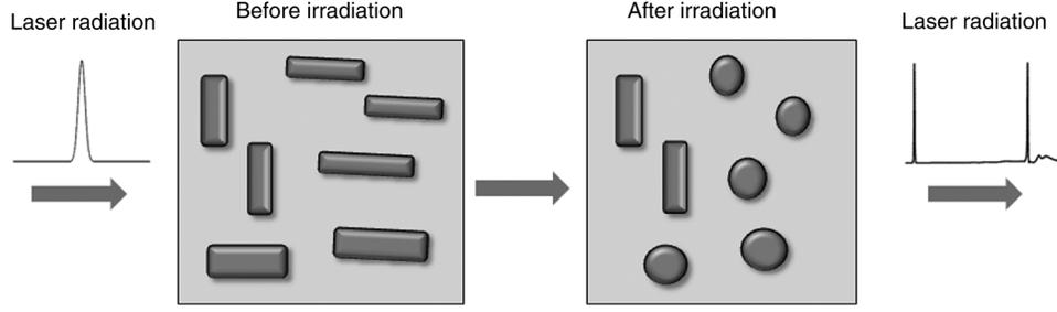
**Fig. 1** Schematic showing of laser radiation interaction with the medium containing nanorods.
