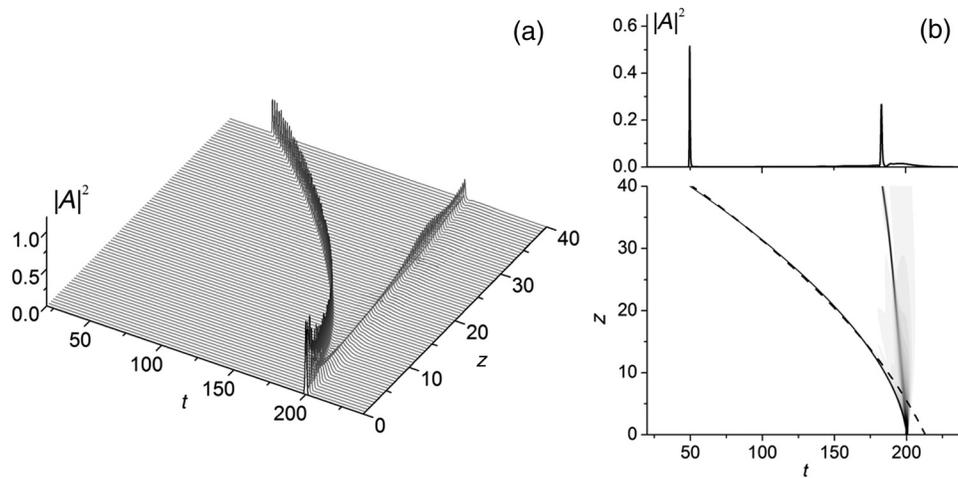
**Fig. 6** (a) Soliton formation and (b) maximal intensity position for both subpulses at the incident Gaussian pulse propagation for the positive phase amplitude grating  $\xi = 5$  and  $\delta_0 = 0.005$ ,  $\bar{\delta} = 5$ . Dashed line in (b) is given by Eq. (47). The top plane in (b) shows subpulse shapes at section  $z = 40$ .
