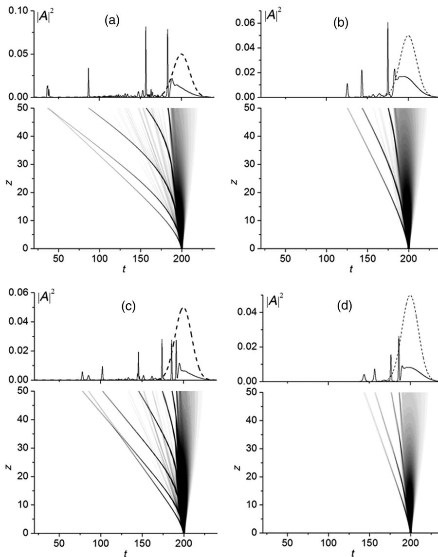
**Fig. 13** Maximal intensity position for subpulses appearing at the incident Gaussian pulse propagation for (a) and (b)  $\delta_0 = 0.05$ , (c) and (d) 0.1, (a) and (c)  $\xi = 2.5$ , (b) and (d) 1.25, and  $\bar{\delta} = 5$ . The top figures show subpulse shapes at section  $z = 50$ . Dashed lines correspond to the pulse propagation in a linear medium.
