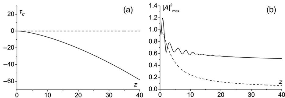
**Fig. 7** (a) Pulse center shift along the  $z$ -coordinate, calculated using Eq. (12) and (b) maximal intensity evolution in a medium with the positive phase amplitude grating  $\xi = 5$ ,  $\delta_0 = 0.005$ , and  $\bar{\delta} = 5$ . Dashed lines correspond to the pulse propagation in a linear medium.
