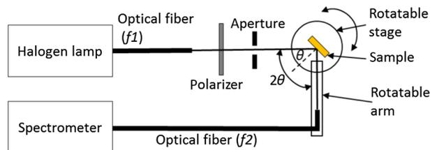
**Fig. 3** Schematic of the custom spectrometer used for reflectance measurements.
