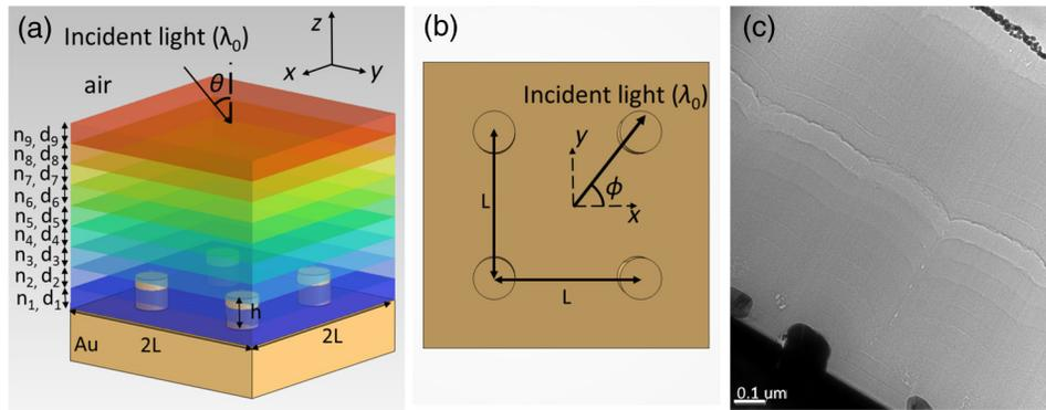
**Fig. 1** (a) Schematic of a one-dimensional (1-D) photonic crystal (PC) deposited on top of a two-dimensional (2-D) metal grating. Only one period of the PC is shown. The wavevector of the incident light is inclined at  $\theta$  with respect to the  $z$  axis, and (b) at  $\phi$  with respect to the  $x$  axis in the  $xy$  plane. (c) Transmission electron microscopy image of the fabricated sample with two periods of PC.
