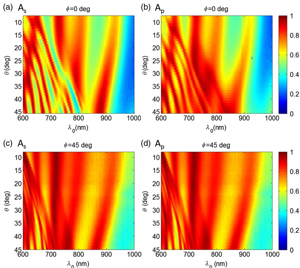
**Fig. 7** Absorptances (a,c)  $A_s$  and (b,d)  $A_p$  of the fabricated structure measured as functions of  $\lambda_0$  and  $\theta$  for (a,b)  $\phi = 0 \text{ deg}$  and (c,d)  $\phi = 45 \text{ deg}$ .
