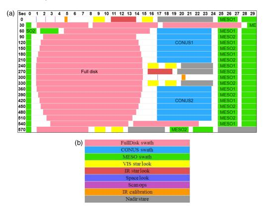
Fig. 5 The diagram of (a) scan mode 6M currently operational for GOES-17 ABI and (b) its scene legend.<sup>29</sup>
