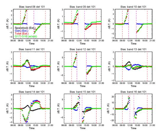
**Fig. 7** The difference between the calibrated BT of GOES-16/GOES-17 ABIs on May 1, 2019, is compared with the estimated GOES-17 calibration bias induced by floating FPM temperature: black: estimated bias induced by SL counts variation; blue: estimated bias induced by gain variation; red: estimated total bias; green: offset observed from GOES-16/GOES-17 comparison. The red vertical lines are the gain switch time. The purple vertical lines bracket the period of ICT look saturation.
