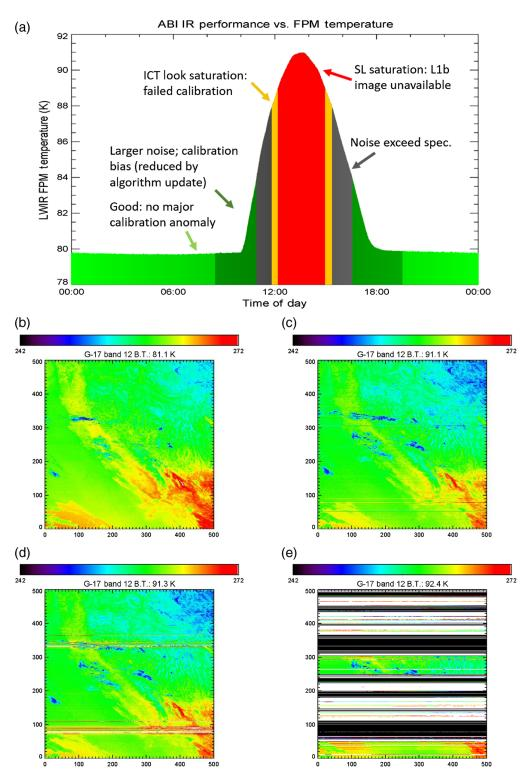
**Fig. 11** (a) A sketch summarizing the dependence of ABI IR performance on the FPM temperatures. The MESOs from (b) to (e) demonstrate how L1b qualities degrade with rising FPM temperatures for a period from 0930 UTC to 1045 UTC on August 28, 2019.
