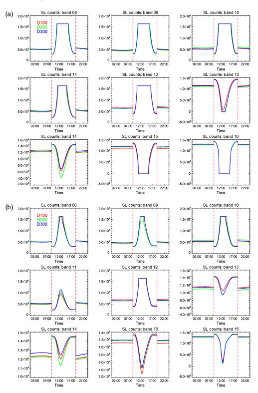
**Fig. 4** The daily profile of SL counts of GOES-17 ABI IR detectors during (a) May 3, 2019, and (b) April 14, 2019. The peak LWIR temperatures are 98 and 108 K, respectively. The vertical red dashed lines represent the time of gain switch.
