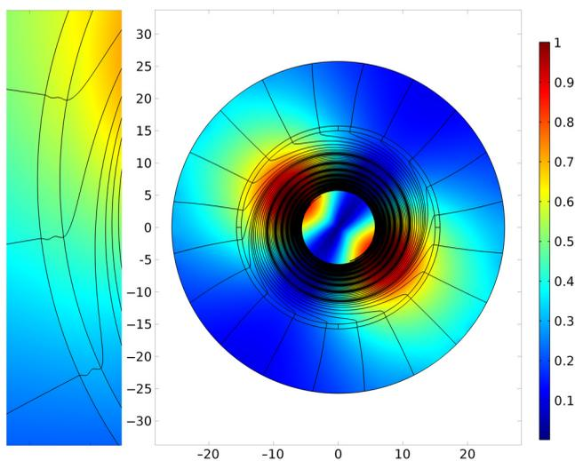
**Fig. 3** Distribution of the transverse Poynting vector component projection on the radius vector direction in the silica glass capillary cross section. The streamlines for the transverse component of the Poynting vector (black lines). All dimensions are in  $\mu\text{m}$ .
