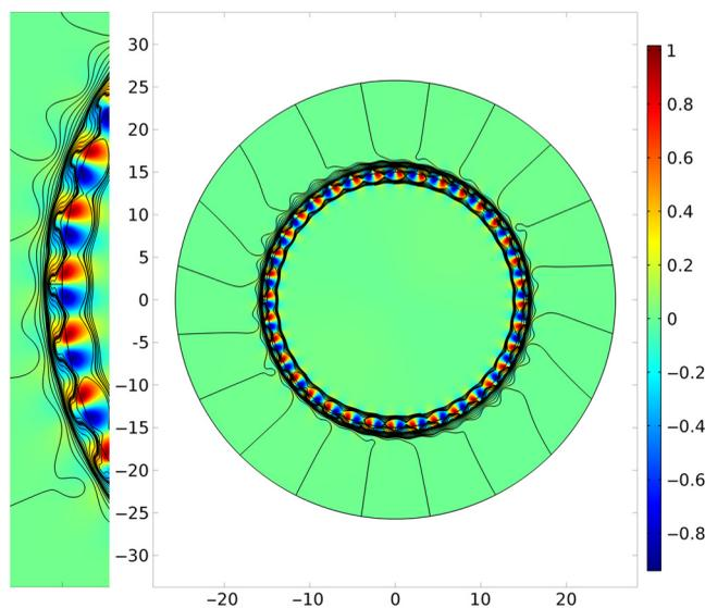
**Fig. 4** Distribution of the transverse Poynting vector component projection on the radius vector direction in the silica glass segmented capillary cross section ( $N = 36$ ). The streamlines for the transverse component of the Poynting vector (black lines). All dimensions are in  $\mu\text{m}$ .
