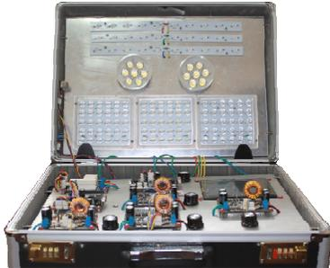
Figure 4. LED lighting system based on capacitive touch and infrared wireless remote control. Figure 5. Project defense scene.
