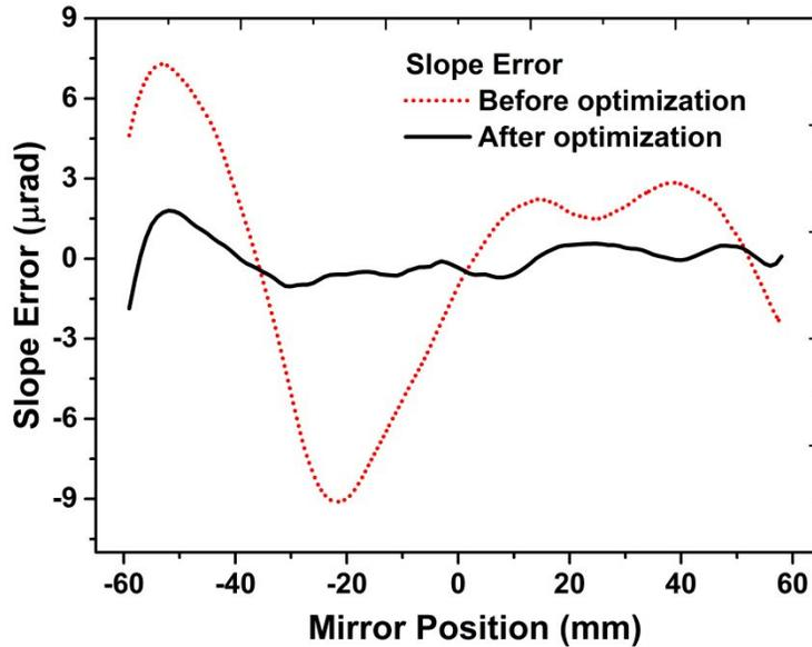
Figure 3. The optical slope error of the bimorph mirror was reduced from 2.3  $\mu\text{rad}$  at zero piezo voltages (orange, dash-dot) to 0.2  $\mu\text{rad}$  (solid, black) at optimized voltages.
