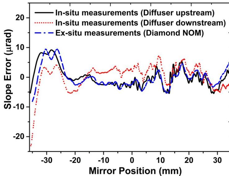
Figure 2. A comparison of the slope error of an elliptical test mirror as measured using: *in-situ* portable device with a diffuser downstream (red, dots); *in-situ* metrology using a diffuser upstream (black, solid); and ex-situ profilometry using the Diamond-NOM (blue, dash).
