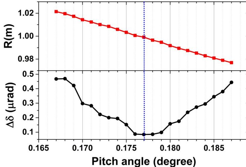
Figure 4. The measured (Top) wavefront radius of curvature ( $R$ ) and (Bottom) corresponding wavefront slope error ( $\Delta\delta$ ) as function of the pitch angle, and the best alignment angle is marked with blue dotted line.
