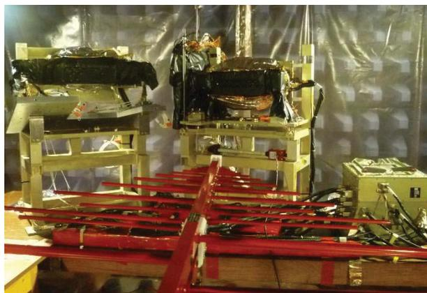
Figure 14: VNIR & SWIR EM FPAs during radiated EMC tests
