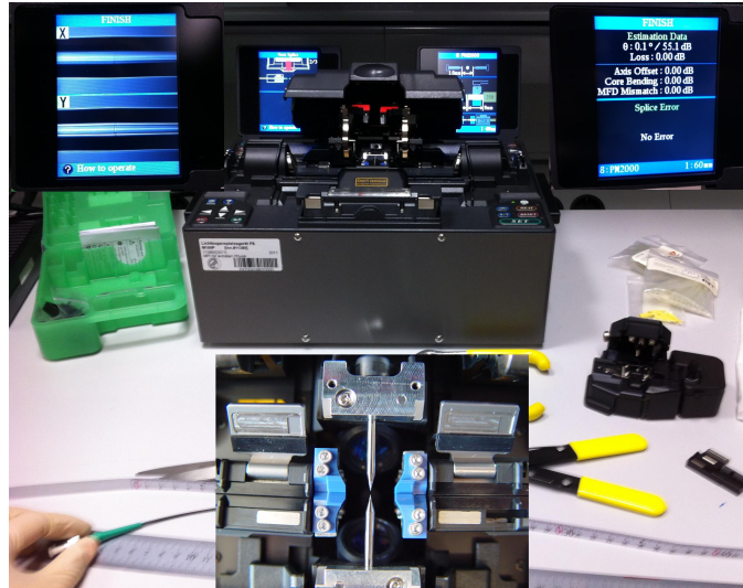
Figure 2. Fusion splicer FSM-100P from the company Fujikura: in the middle the device is displayed with open lid. The surrounding three close-ups show the two displays with the result of a successful splice and the electrodes which perform the fusion splice. The fibers are placed in fiber holders next to the electrodes for this purpose. The left display shows the camera inspection of the splice in perpendicular x and y view. The right display summarizes the quality parameters of the splice with the angle of alignment and the corresponding extinction ratio. 1
