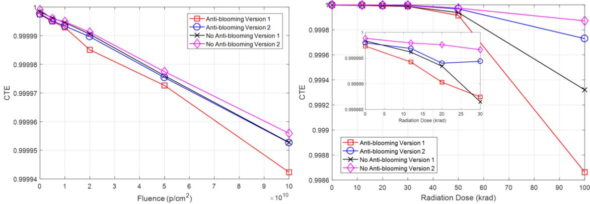
Figure 10 CTE versus Proton fluence (left) and Gamma dose (Right).
