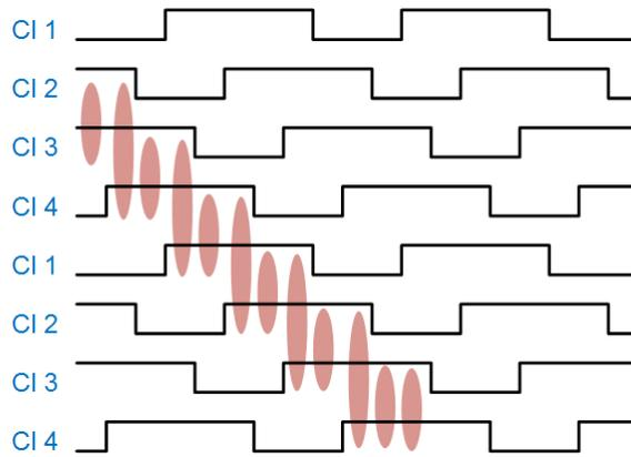
Figure 2: CCD structure phase clocking.
