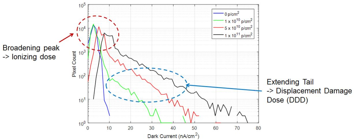
Figure 10 Bright pixel post proton and 14 days room temperature anneal.
