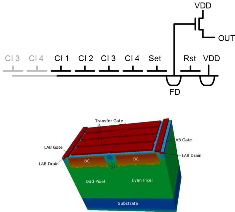
Figure 1 Pixel schematic and 3D structure.
