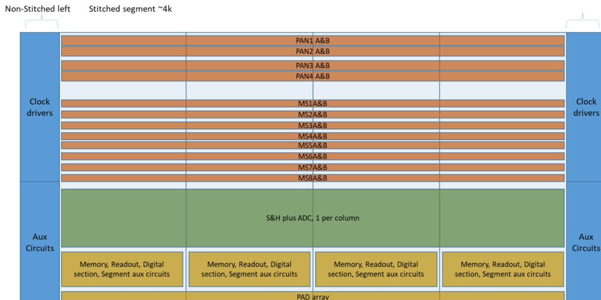
Figure 11 Sensor Architecture
