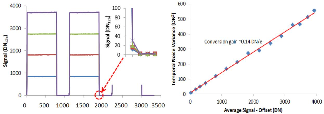
Figure 7 Left CTE measurements and right Photon Transfer Curve.
