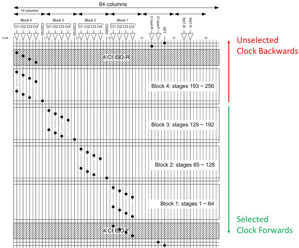
Figure 6 CCD structure phase clocking.
