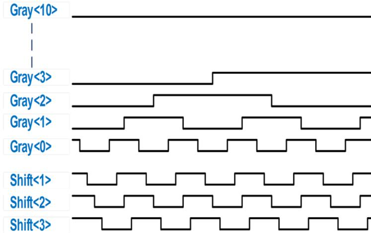
Figure 4 Example of timing access to the sensor CIS125.
