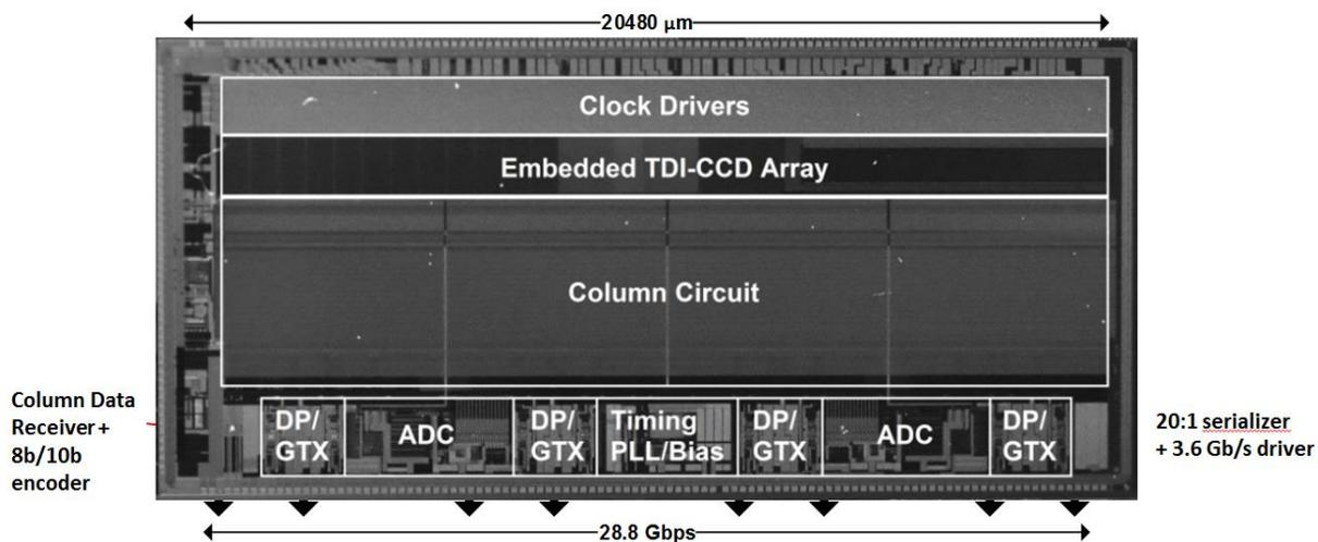
Figure 3 Die design prototype
