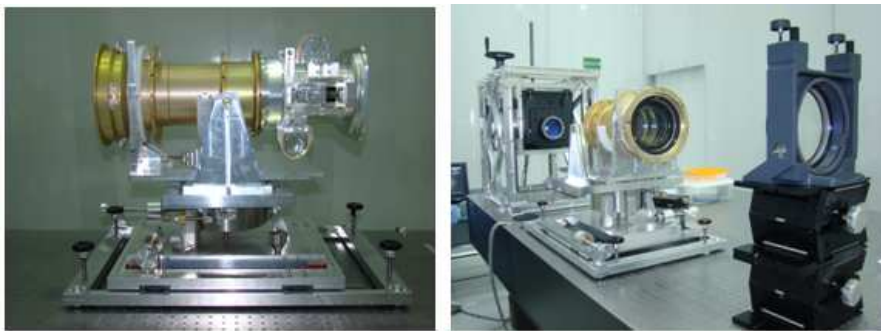
Fig. 4. Collecting lens with focus adjust lens assembled in alignment stage.
