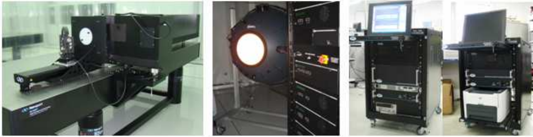
Fig. 1. Some of the equipments of the Ground Support Equipments: collimator, integrating sphere, GSE controller, and image display system (Courtesy Opto Eletrônica S.A.).
