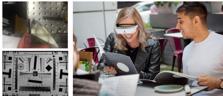
Figure 5 A high-resolution freeform-eyepiece (Left) enables the development of a wearable display as an assistive technology (Right) for people with compromised vision (Credit for Photo on the right: eSight Corporation)
