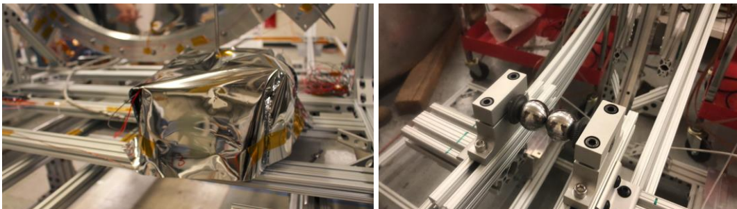
Figure 7. (left) The inflation unit wrapped in Mylar and Kapton to prevent it from directly radiating heat to the membrane and (right) One of three tooling balls that were used to ensure the membrane was inflated to a repeatable mechanical datum.
