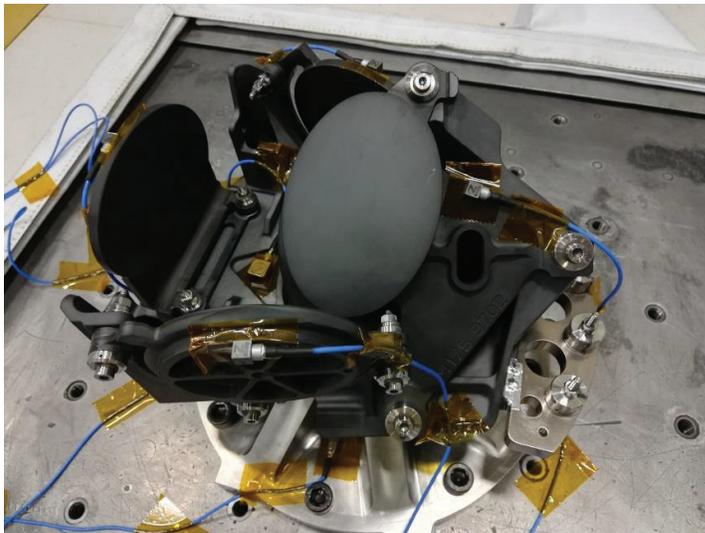
Figure 12: Derotator (STM) installed and instrumented on shaker table.
