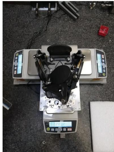
Figure 13: Derotator (STM) mass properties measurement.
