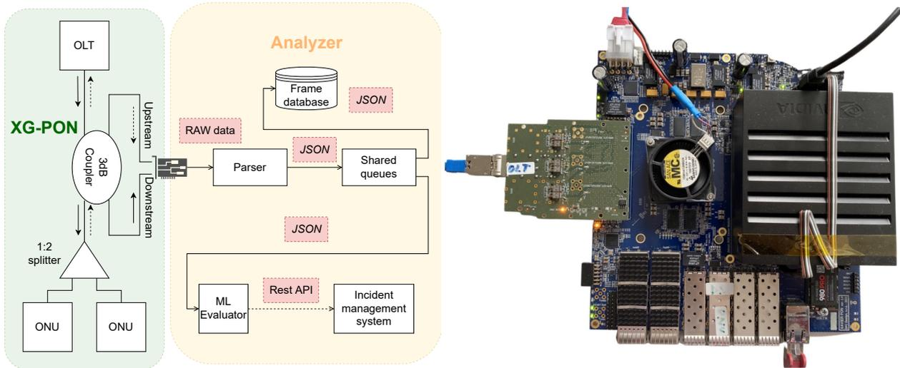
Figure 1: (a) Schematic diagram of the proposed analyzer deployed in a real XG-PON. (b) Newly designed FPGA-based network interface card used for XG-PON frame capturing.
