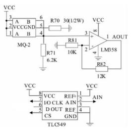
Figure 14. LM358 wiring diagram
