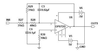
Figure 15. Second order infinite gain low-pass filter circuit
