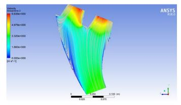
Figure 8. Vortex diagram of pressure stabilizing chamber
