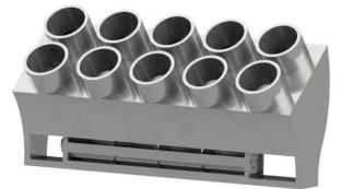
Figure 7. Model diagram of pressure stabilizing chamber and air supply device
