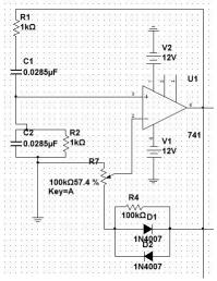
Figure 13. RC bridge sine wave oscillation circuit
