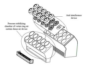
Figure 6. Structure diagram of module core design
