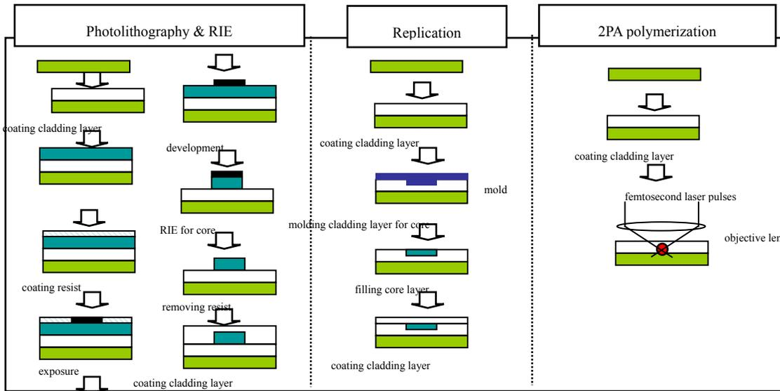
Figure 2 Optical waveguide fabrication methods
