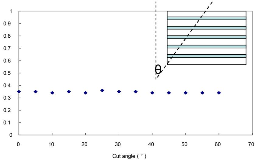
Figure 6 Cut angle dependence of insertion loss of cut waveguide.
