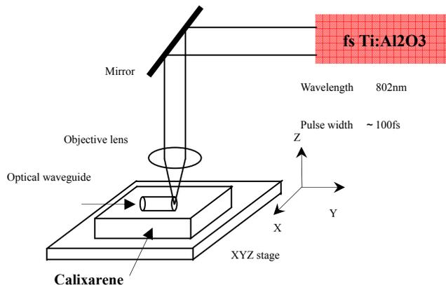
Figure 3 Experimental set-up of TPAP method
