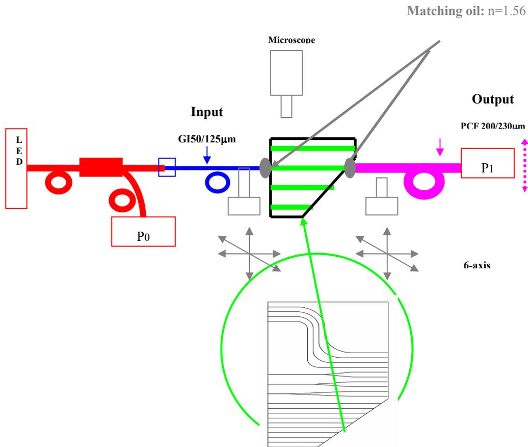
Figure 8 Measurement set-up for optical waveguide chip
