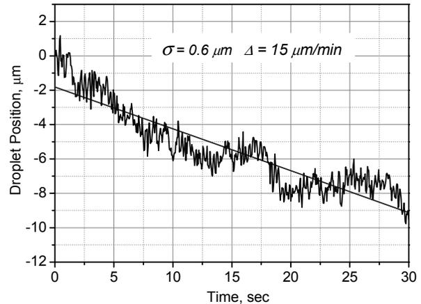
Figure 15: Horizontal position stability of 50 μm droplets.
