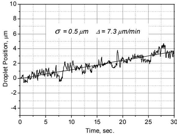
Figure 14: Vertical position stability of 50 μm droplets.
