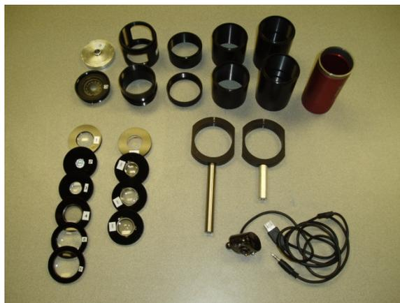
Figure 2. Components of the lens design kit.
