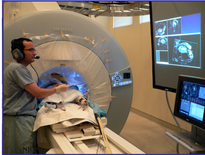
Figure 1. Interventional cardiac MRI suite employing a modified clinical scanner with a shorter bore and a wider opening. Image adapted from McVeigh et al. Springer © 2008.
