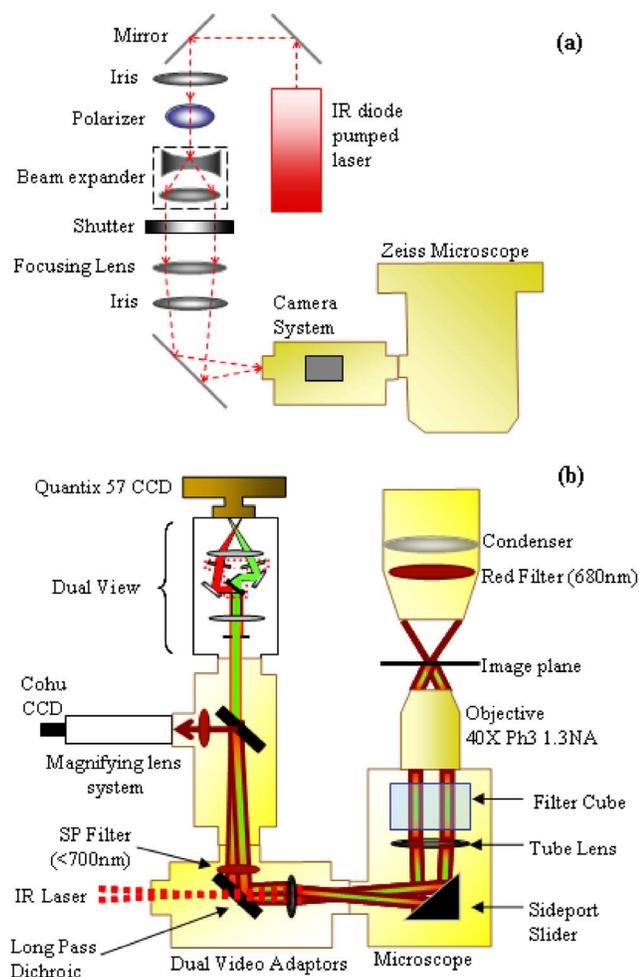
**Fig. 1** (a) Optical schematic showing the optical components used to generate and control the laser tweezers and (b) imaging setup showing the illumination sources, filters, and cameras used to image the sperm in both phase contrast and fluorescence.
