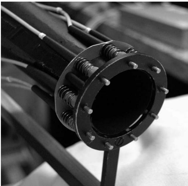
**Fig. 2** Emitting fibers located on the ring, spring mounted independently.
