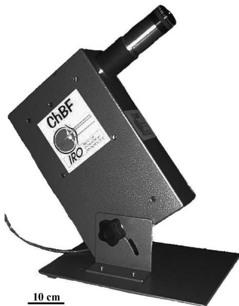
Fig. 3 Photo of the compact confocal choroidal flowmeter.
