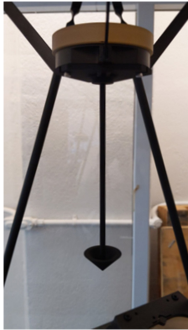
Fig. 18 The conical baffle is fastened onto the FC1 mounting ring and sits beneath the field corrector assembly.
