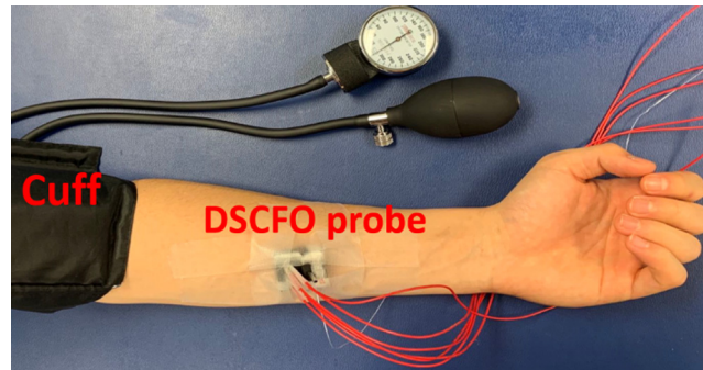
Fig. 4 DSCFO measurements of \Delta[\text{Hb}] , \Delta[\text{HbO}_2] , and rBF in the forearm during artery cuff occlusion on the upper arm. A wearable DSCFO probe was fixed on the forearm using medical tapes. An inflatable cuff was installed on the upper arm for artery occlusion.
