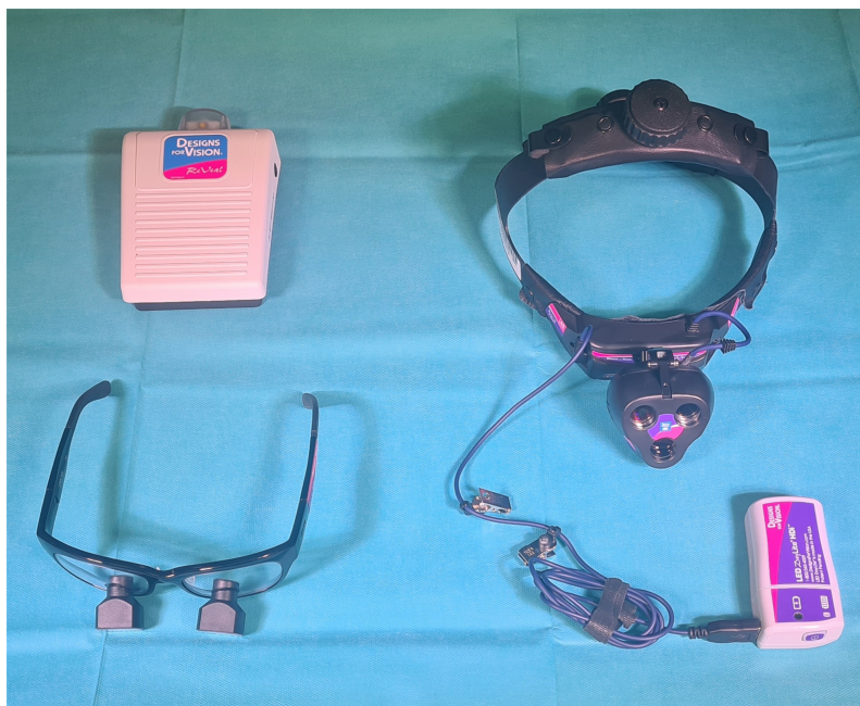
Fig. 1 Illustration of the loupe device used within this study. All essential intraoperative components of the novel loupe device are shown. The specifically developed headlight (top right) is wired to a rechargeable battery pack (bottom right). The remote paddle (top left) allows the surgeon to easily toggle between illumination modes, while the surgical goggles (bottom left) feature specific filters that facilitate conventional white light surgery as well as adequate and safe visualization of 5-ALA induced fluorescence.
