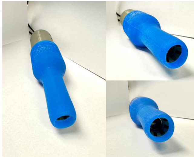
Fig. 7 PPRIM prototype system with a flexible sheath. The main body casing is shown inserted into the flexible sheath.
