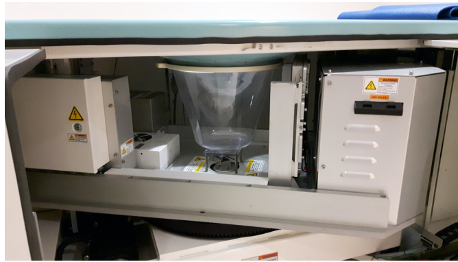
Fig. 25 Photo of a flat panel cone beam dedicated breast CT system showing the main components of the imaging chain. The plastic cup located surrounding the space for the pendant breast isolates the moving parts of the system from the breast and the rest of the patient.
