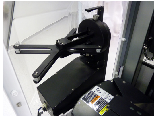
Fig. 2 Wafer flipper used to facilitate the imaging through the back-side of wafers.
