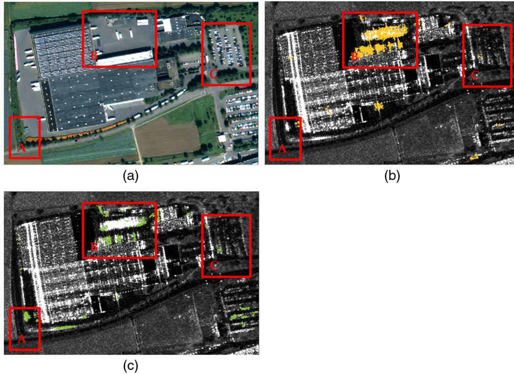
Fig. 22 Results of HAO assignment utilizing z = 50 . (a) WV-2 image subset, (b) assignment result for final class 3 (construction site) as overlay on time series mean amplitude image. (c) Assignment result for final class 5 (collecting point). (A) Container collecting point, (B) mixed area of collecting points and loading/unloading points, (C) car parking lot. The color-coding of the high activity pixels refers to Fig. 20 or Fig. 21.
