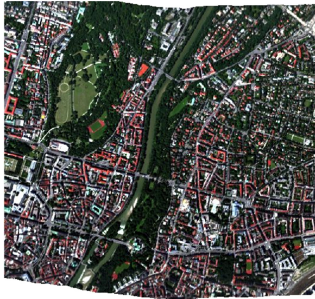
Fig. 2 HyMAP true-color image of the Isar River, Munich, Germany (R: 635 nm, G: 543 nm, and B: 466 nm).
