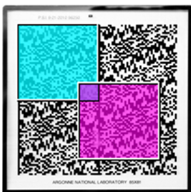
Fig. 3 An extended Hadamard mask of size 81 \times 85 pixel fabricated on a quartz plate with chrome coating. A 41 \times 43 pixel mask area such as the ones indicated by the colored boxes is exposed for each acquisition.
