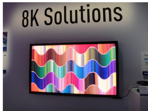
Fig. 16 55-in. 8K4K display realized color gamut covering 99% ( u'v' ) of BT.2020 with the laser diode in International CES2016: we collaborated with the connection technology of plastic optical fiber. 19
