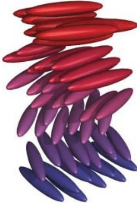
Fig. 2 A representation of a cholesteric liquid crystal (also known as a chiral nematic liquid crystal) that is structurally chiral. Adjacent liquid crystal molecules are twisted relative to their neighbors. (Courtesy of Kevin G. Yager, National Institute of Standards and Technology, Gaithersburg, MD, USA.)
