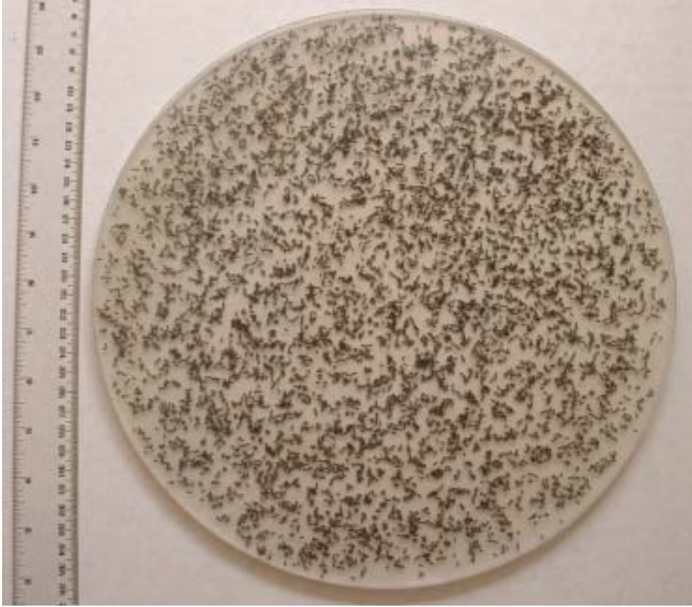
Fig. 3 An isotropic chiral material fabricated for microwave applications. Miniature springs are randomly dispersed in epoxy. (Courtesy of Álvaro Gómez, Universidad de Cantabria, Spain.)
