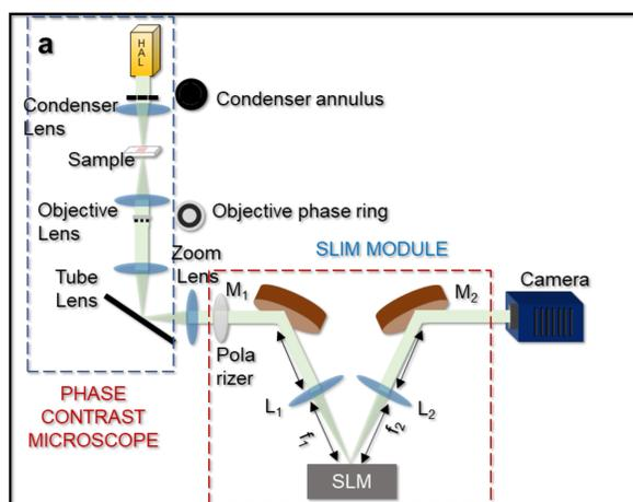
Fig. 1 Spatial light interference microscopy (SLIM). Figure Courtesy. Ref.11
